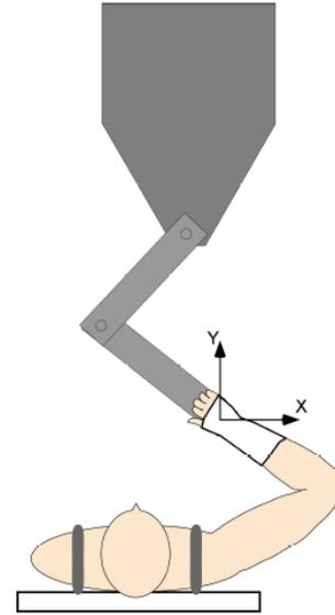
Fig. 1. Robotic device for evaluate end-point stiffness
